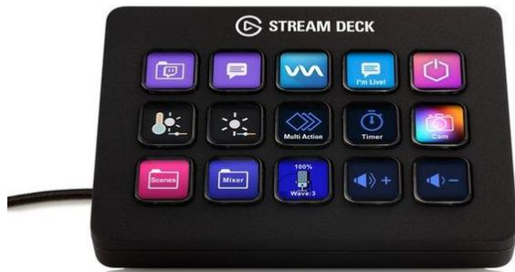
The Elgato Stream Deck can control many popular software programs and it would be a great way to trigger commands to be sent to radios and station accessories. The Stream Deck button can be programmed to send a specific command to the macro.exe program which, in turn, sends a command out a serial port to the target device. A more flexible approach would be to send a macro name to the macro.exe program which, in turn, sends one or more commands to one or more serial ports.
