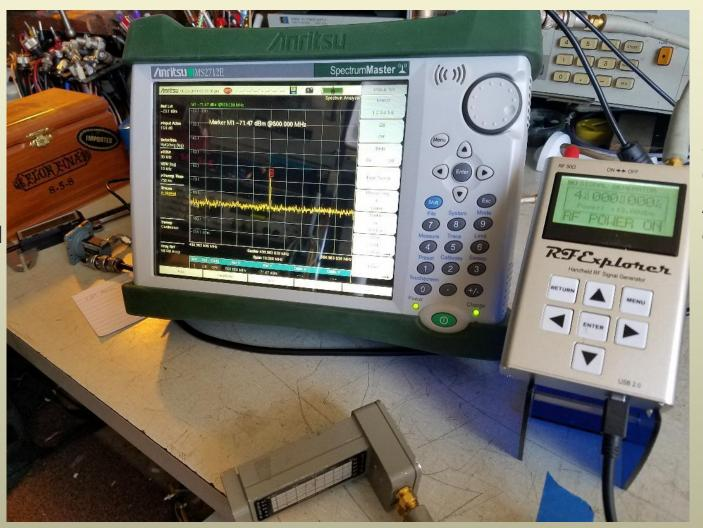
Signal Generator At 4GHz 8mw
